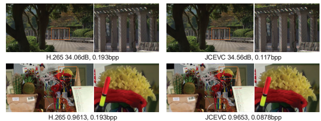
Figure 1: Reconstructed frames with H.265 (x265 LDP very fast) and JCEVC. The JCEVC achieves a significantly higher RD performance than H.265 by reducing bit-per-pixel (bpp) almost half whilst retaining competitive PSNR or MS-SSIM.
